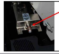
Clean this valve with a soft brush before reattaching the milk frother to it.
