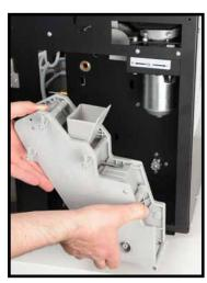
The group needs to be submerged in hot water for 20 minutes, then thoroughly rinsed to remove any coffee grounds.
